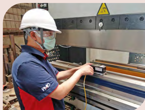
An inspector conducts a type certification inspection of power driven punching-shearing machinery.
