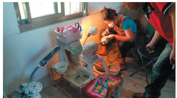
持研磨機手工研磨，旁有窗戶通風，員工配戴口罩
