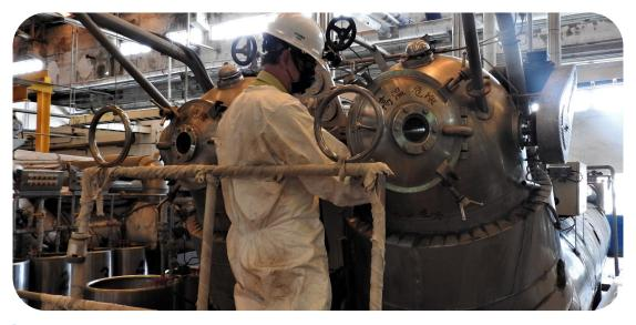
An authorized inspector agent tests the thickness of a Class 1 pressure vessel and inspects its weld beads.
