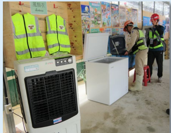
© Mobile water-cooled air conditioners and fan-cooled workwear help lower temperatures.
